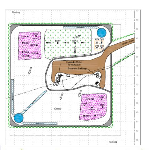
2,750 m<sup>3</sup> of lift #1 was stripped and placed into stockpiles complying with either surface soil or subsoil criteria.
