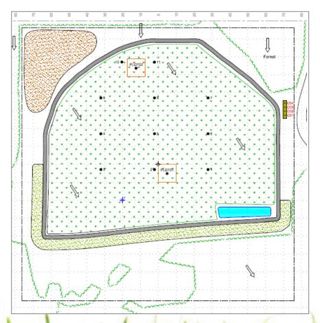
12,000 m<sup>3</sup> of material excavated from 2 former DWDAs, wellbore area, and disturbed area were spread to a depth of 1 m:
