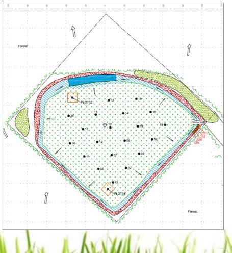
10,000 m<sup>3</sup> of material excavated from a former drilling waste disposal area and earthen pit were spread to a depth of 1 m:
