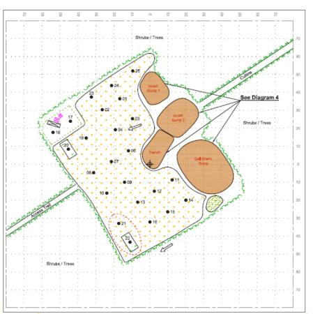
Approximately 5,800 m<sup>3</sup> of material excavated from former pits and sumps onsite to be treated for PHC contamination resulting from historical drilling activities:
